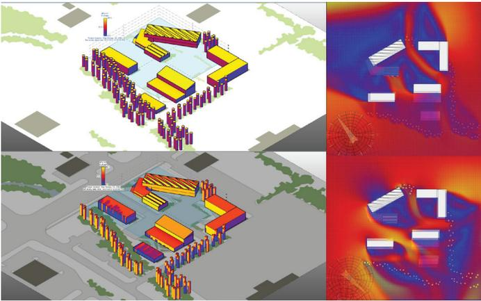
Figure 3. Site development using solar radiation and wind analysis tools (Adrienne Nelson, Amanda Havel and Melissa Goodwin).
