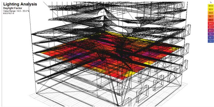
Figure 1. Daylight analysis for one floor level in Rhinoceros / Autodesk Ecotect to understand how a 3 dimensionally distorted courtyard enriches the daylight uniformity of internal spaces (Suncica Jasarovic, ARCH 490, Spring 2012).
